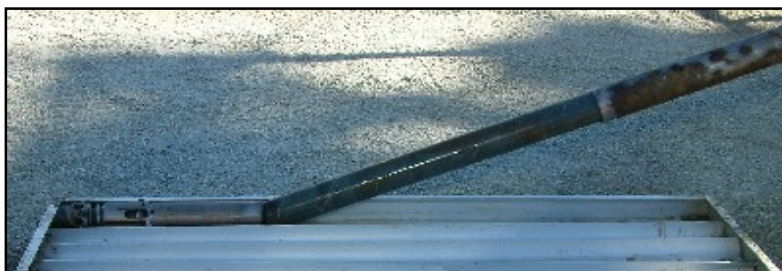
The Ezy-Mark head comes out with the core at the end of the run.
