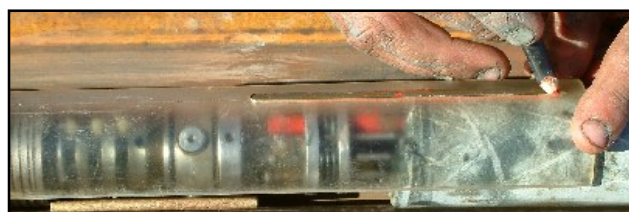
The gauge is aligned with the three orientation balls and the core is marked.
