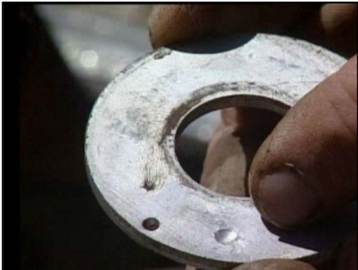
As the core is broken, a non-magnetic ball indents the aluminum disc, corresponding to the bottom of the hole. The pin location is the second (fixed with respect to the core barrel) point of reference used in determining the orientation of the core.
