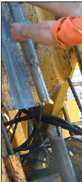
Ezy-Mark lowers down with the core tube.
